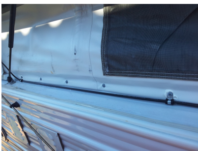
Clip airline neatly into place Use corner fittings at each corner 'Y' fitting & bulk head fitting
