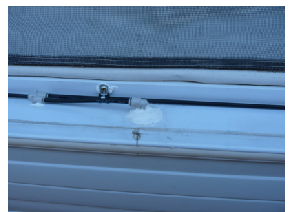
Clip airline neatly into place Use corner fittings at each corner 'Y' fitting & bulk head fitting
